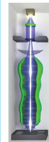
Fig 1. Image of a point-source generated with an aberration free high-NA optical system for a full, reduced and annular pupil.
