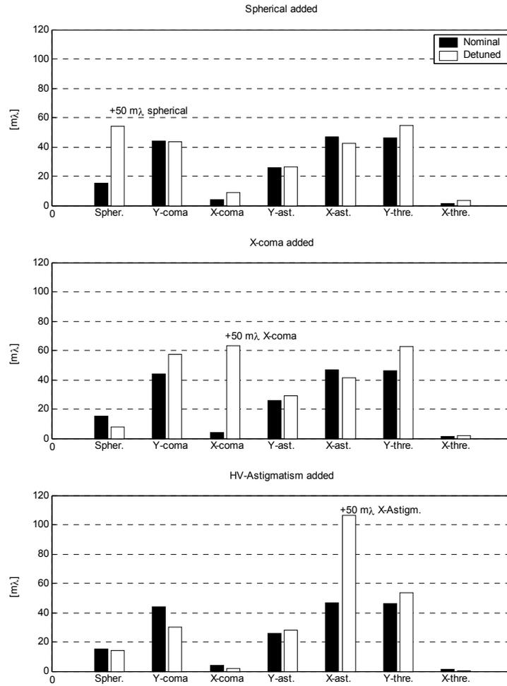
**Figure 2:** Bar diagrams of the measured change in aberration value for three specific aberration types (spherical aberration, coma and astigmatism) using the retrieval method according to the Extended Nijboer-Zernike theory. The black bars indicate the reference aberration values, the white bars the values corresponding to the detuned systems (all values in units of  $m\lambda$  rms aberration).
